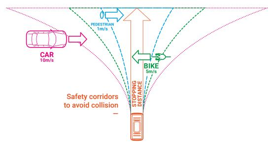
In order to guarantee that a collision won't occur with a pedestrian in this worst-case scenario we have to define a "safety corridor" around the trajectory. The width of this corridor depends on the hypothesis we pose about pedestrian's speed when it crosses.
